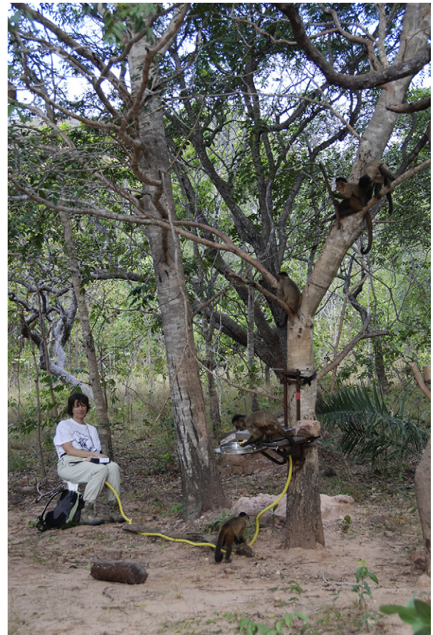
Figure 1. Capuchins' weights were obtained using a mounted scale. The scale was mounted 1 m above the ground with water and food provisioned at the distal end. An experimenter, seated a few metres away, recorded the weight showing on the digital display when one capuchin was fully supported by the scale. Photo: T. Pickering.
